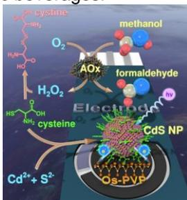
Figure 1: Electrochemical detection of CdS QDs “wired” by an Os-PVP complex to the surface of a screen-printed carbon electrode.
